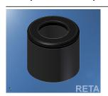
Code1889Cxx Complete rubber spring constituted by rubber spring in rubber and Washer in PA 6. Standard hardness 50 Shore. Available in various Lengths (currently 32, 27, 19, 21). Only rubber thermoplastic adherent to all the norms. NO PVC. The double minuscule x in the code serves to indicate the length. Black color
